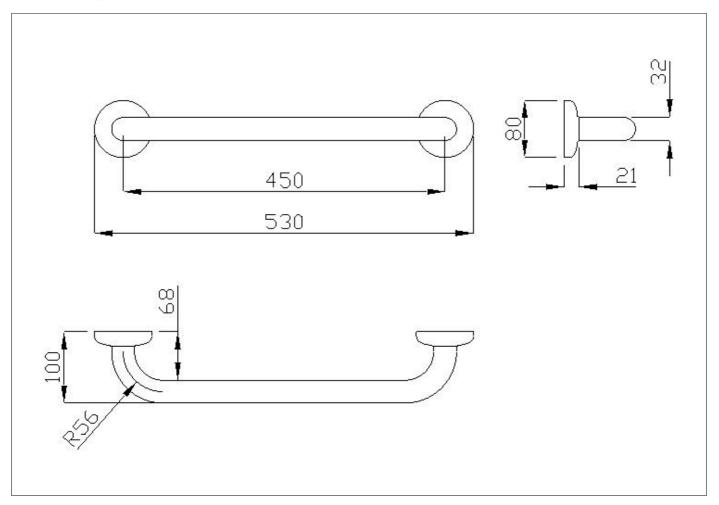
Straight grab bar made of seamless steel pipe, painted with synthetic thermoplastic powder of plant origin,  $Rilsan \circledR$
