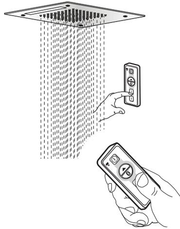
**Note:** a remote control can be associated to several showerheads to control them at the same time. It is not possible, on the contrary, to control a single showerhead with several remote controls.
