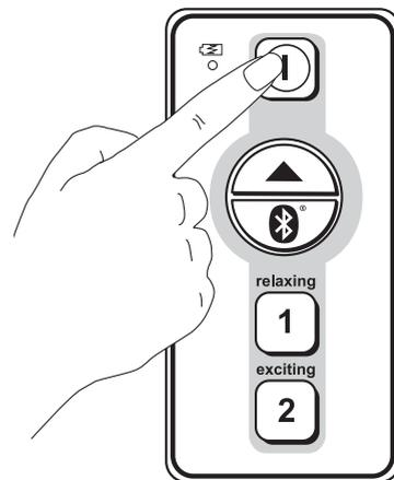
**The remote control is designed according to power-savings guidelines; it switches itself off automatically after 10 seconds non-use; in order to start it again, touch the key again.**
