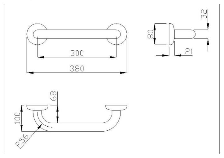
Straight grab bar made of seamless steel pipe, painted with synthetic thermoplastic powder of plant origin, Rilsan®
