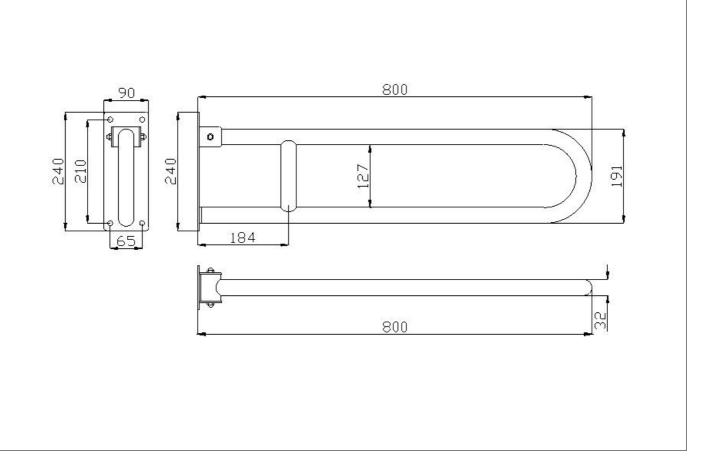
Folding grab bar made of seamless stainless steel AISI 304 pipe, with satin finish
